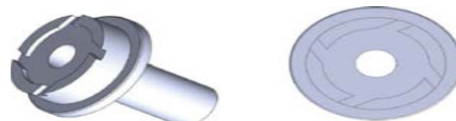
Fig 4 Section of Vortex Tube Inlet Nozzle
